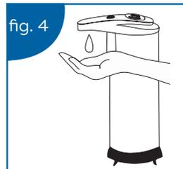
**6.** After turning on, the dispenser volume defaults to 1, the smallest dispensing amount. The volume setting can be adjusted by clicking the on/off button. Each click advances the volume from 1 to 2 to 3, then back to 1. A pause is required between clicks. After clicking, a red light blinks to the following patterns to confirm the new volume setting;
